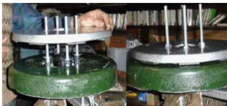
Fitting the front magnet rotor
